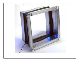
Metal duct is another path for structureborne sound transmission. Canvas connectors should be used to break the metal to metal contact and eliminate this transfer path. This is noted in the Installer's Guide:
