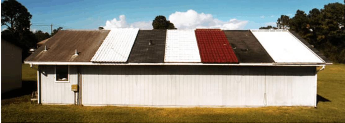
**Figure 2. FSEC Flexible Roof Facility showing roof/attic test cells under test. The 2 test cells with the dark composition shingle roofs are the subject of this report.**
